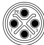
3+PE-pos. S-coded for power supply
